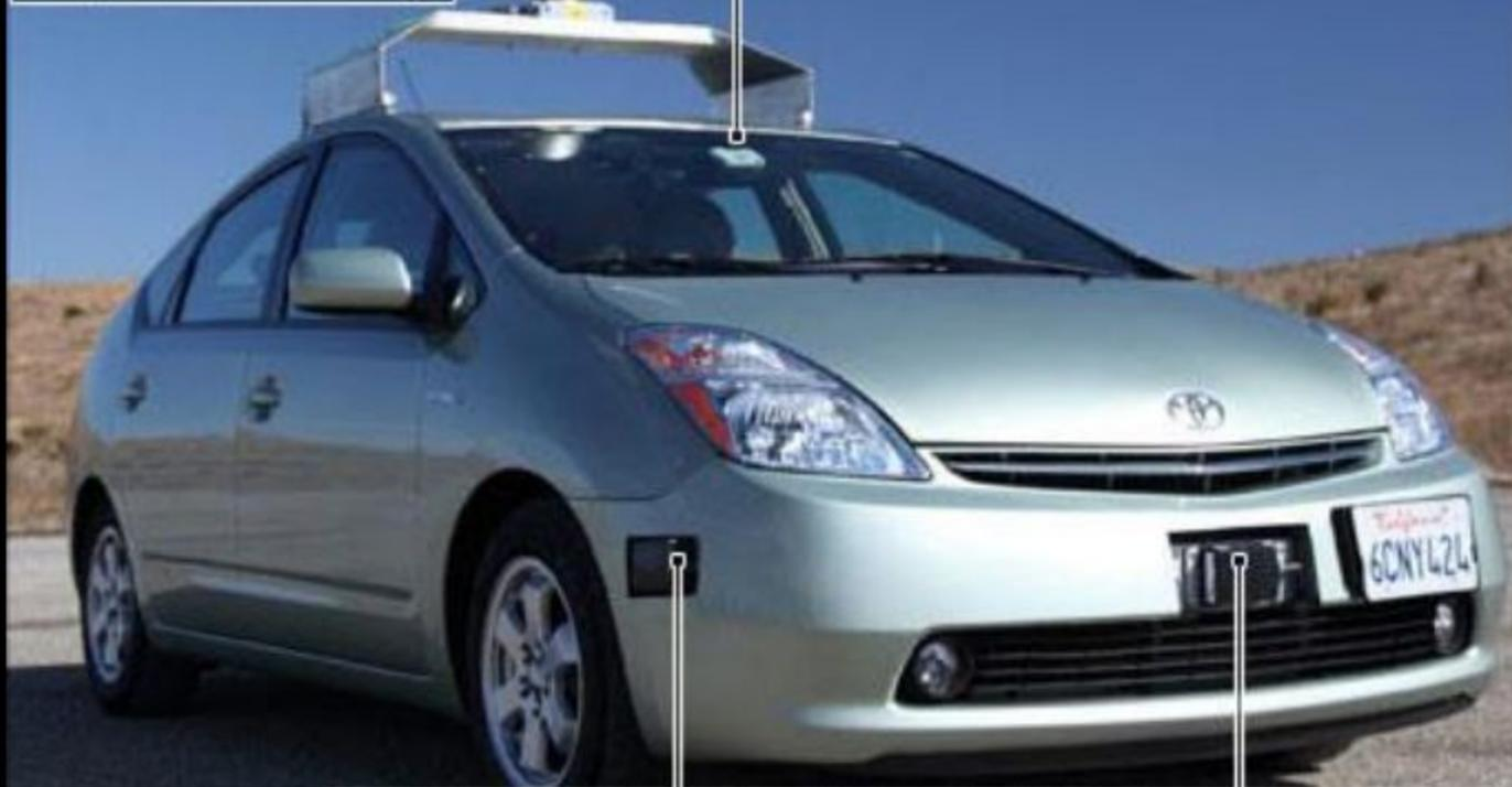
**Radar sensors - three at the front and one at the back - help determine position**
